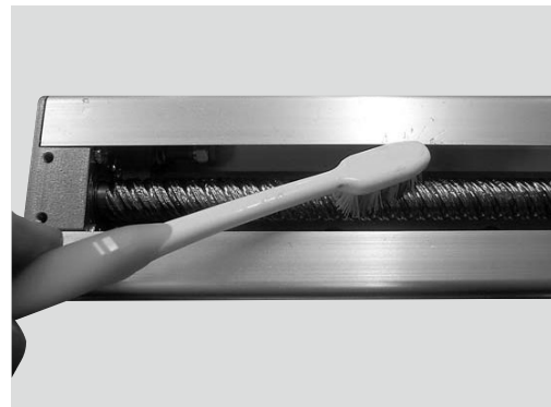
Applying grease to the ball screw
