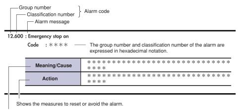
Shows the alarm meaning and the cause of the alarm occurrence.
