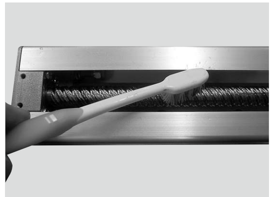
Applying grease to the ball screw
