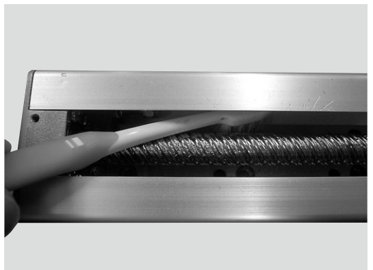
Applying grease to the linear guide
